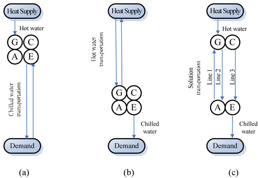
FIG. 2. Concept of sensible heat transportation [4]
