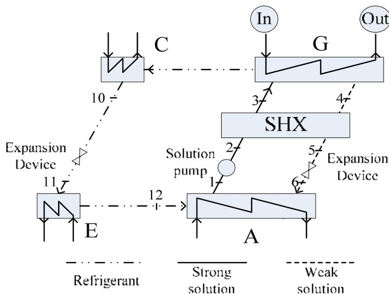
FIG. 1. Schematic diagram of a single effect absorption cycle [6]
